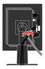
Remove the Rubber Cover from the back of the stand. And then replace the Cable Cover.
